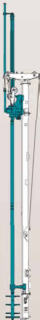
SOIL MIXING Depth/Hloubka 25 m Ø 1000mm
